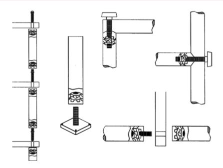
Inside Tube Diameter = 24,6-25,6 Outer tube diameter = 1 1/8" Thread = M8
